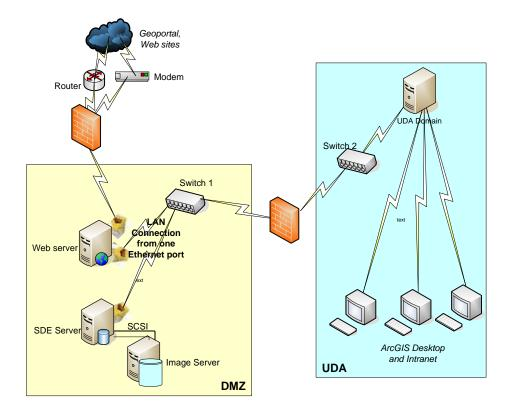
Figure 2. 7 Scheme of architecture for DMZ zone and UDA network
