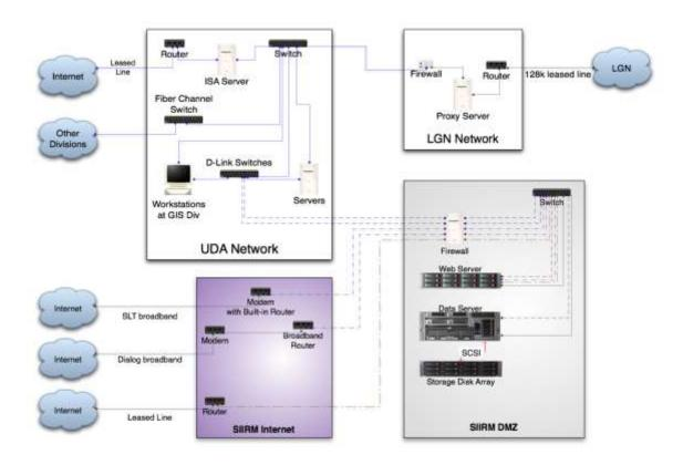
Figure 2. 8 Scheme of final network architecture
