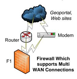
Figure 2. 5 Configuration with Internet connections and multi-WAN firewall
